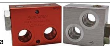
These valves are ideally suited for unidirectional motor applications when using a control valve that has closed work ports in the neutral position. The cross port check valve permits the centrifugal energy of the driven component to dissipate harmlessly.
