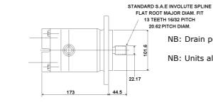
NB: Drain port must be connected to tank
