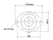
OIL INLET AT A - SHAFT ROTATION RIGHT OIL INLET AT B - SHAFT ROTATION LEFT
