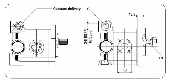
NB: Constant flow rate must be stated with order. Example pump code with 'P2' option and 8 Lt/Min constant flow at 'C'. PLP20-20-82E2-GEGD-P2-8
