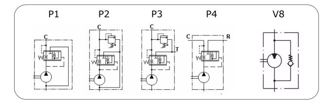
P1 = Constant Flow at 'C'; Excess flow to inlet.
