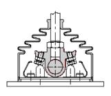
**07 Control** - Detent in position 1 and 2, spring centred to neutral position.
