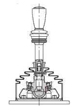
**11 Control** - Detent in positions 1 and 2. Detent in neutral, lift to release.
