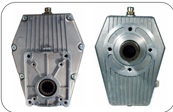
Designed to adapt the Casappa Group 3 PLP30 range of gear pumps to the power take off of an agricultural tractor by providing a speed increasing ratio.
