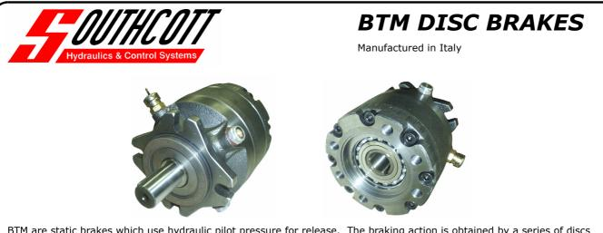
BTM are static brakes which use hydraulic pilot pressure for release. The braking action is obtained by a series of discs and springs acting onto the main piston. The brake housing is of spheroidal cast iron and extrusion proof seals are suitable for high pressures.
